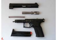
No further disassembly is needed for routine maintenance. When a great number of cartridges has been fired, it is advisable to have the firing pin and magazine cleaned by a competent gunsmith.
